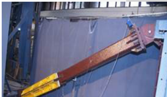
In Image: Full-scale hybrid buckling-restrained brace.
